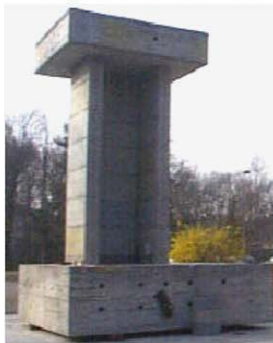
Fig. 10. U-shaped wall: description of the specimen and loading history.
