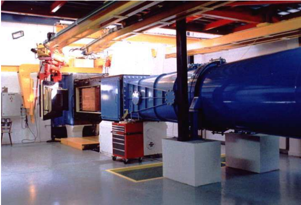
Fig. 1. View of the S3Ch wind tunnel of the ONERA Meudon centre
