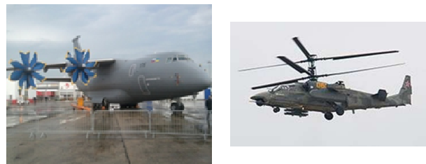
Fig. 1. Dual-rotor co-axial configurations. Left: Antonov-70 with contra-rotating propellers. Right: Kamov-52 with co-axial rotors
