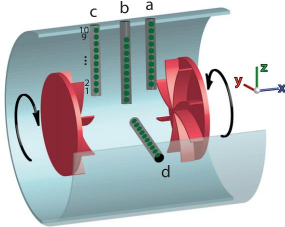
**Figure 1.** Experimental setup showing the location of the Hall probes, where  $x$  is the axial coordinate directed from impeller 1 to impeller 2.
