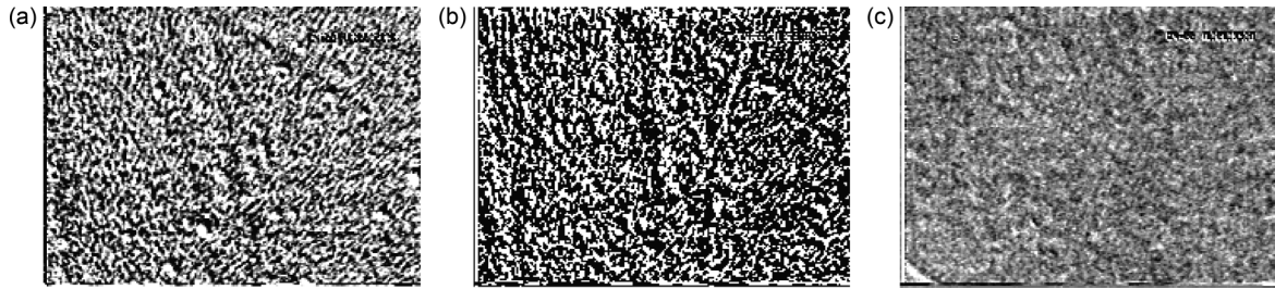
FIG. 2. Enhanced bright field (a), phase contrast (b), and dark field (c) images taken at approximately 1 mK above the critical temperature. The images are single frames extracted from video recorded at 25 frames/s and the correlation length at this temperature was \approx 1 \mu\text{m} . The height of the image is 1.5 mm.
