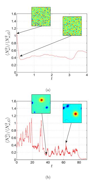
FIG. 3: Evolution of the ratio of the total mean square nonlinear term in turbulent flow to the equivalent value in the Gaussian flow for short times (a) and long times (b). Snapshots of the vorticity field are shown for four different time instants. In the top figure these snapshots only show a quarter of the domain to more clearly identify the flow structures. Results correspond to the 1024<sup>2</sup> run.
