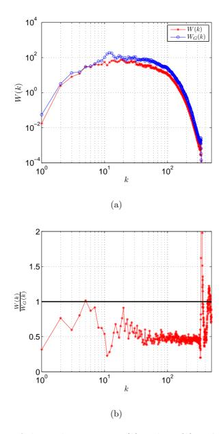
FIG. 6: Top: spectrum of the nonlinear term W(k) and  $W_G(k)$  evaluated at t=4. Bottom: normalized power spectrum  $W(k)/W_G(k)$  of the nonlinear term evaluated at t=4.
