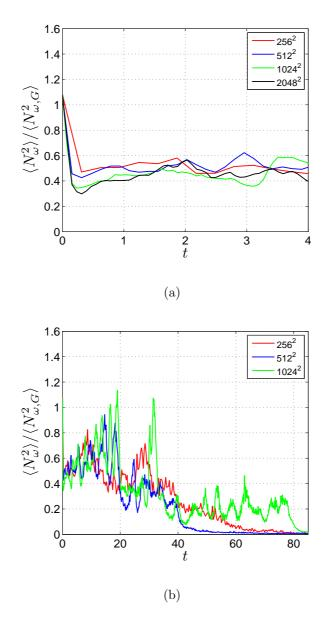
FIG. 7: Evolution of the ratio of the total mean square nonlinear term in turbulent flow to the equivalent value in the Gaussian flow for short times (a) and long times (b).
