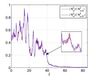
FIG. 4: Evolution of the ratio of the total mean square nonlinear term in turbulent flow to the equivalent value in the Gaussian flow. The turbulent statistics for the  $512^2$  run are compared to two independently generated Gaussian fields  $\langle N_{\omega,G}^2 \rangle$  and  $\langle N_{\omega,G^*}^2 \rangle$  to check the influence of the choice of the Gaussian fields on the results.
