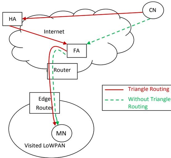
Figure 2: Communication between the mobile node and its correspondent through triangle routing process
