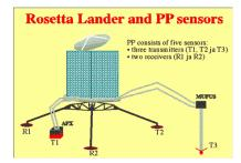
Figure 1: Sketch of the five electrodes used by PP.
