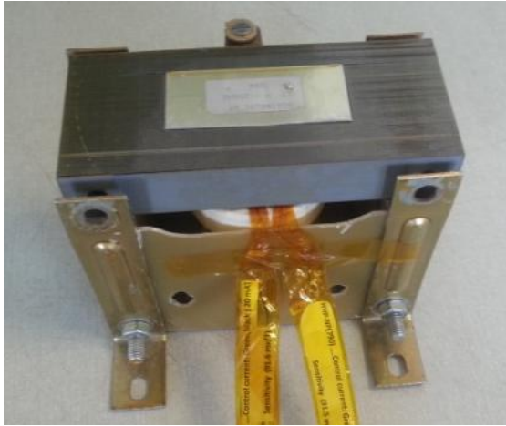
Fig. 7. The realized iron core for the experiments.
