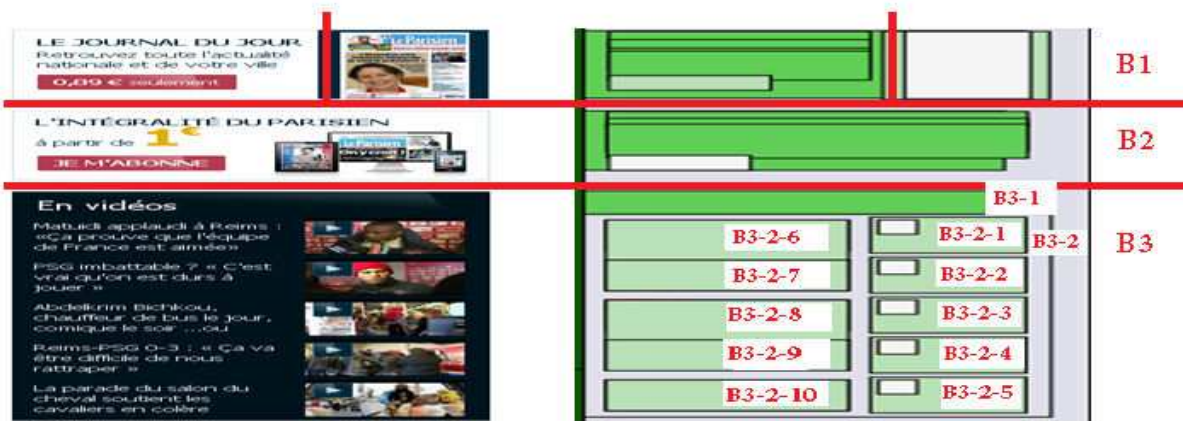
(a) A part of a web page (b) Vision-based segmentation Figure 1. A part of a web page (leparisien.fr) and its vision-based segmentation
