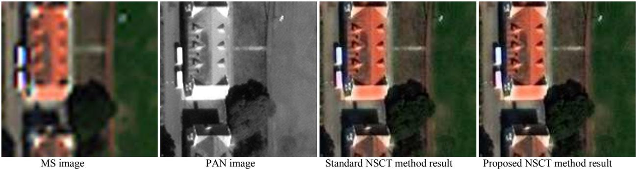
Fig. 10: NSCT-based pan-sharpening.
