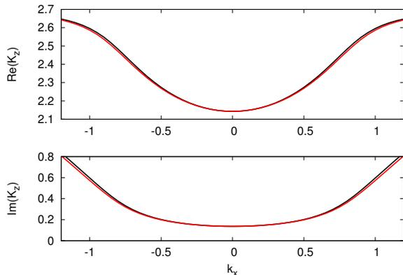
FIG. 2. Dispersion curves for a metallo-dielectric structure ( $h_d = 33.7$  nm,  $h_m = 28.1$  nm,  $\lambda = 363.8$  nm) presenting an effective index close to  $-1$ . Top: Real part. Bottom: Imaginary part. The local (black line) and nonlocal (red line) cases are shown. Very little difference can be seen, especially close to normal incidence.
