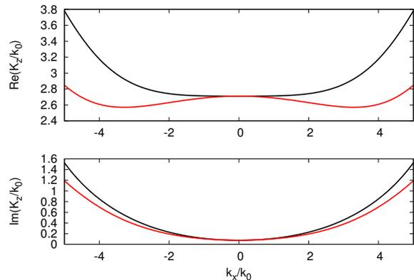
FIG. 3. Dispersion curves for a metallo-dielectric structure ( $h_d = 5$  nm,  $h_m = 22.6$  nm,  $\lambda = 363.8$  nm) in the canalization regime (*i.e.* a flat dispersion curve). Top: Real part. Bottom: Imaginary part. The local (black line) and nonlocal (red line) cases are shown. The difference is much more important here: nonlocality has a direct impact on the curvature of the dispersion curve.
