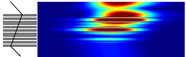
FIG. 5. Propagation of an incident Gaussian beam with a waist of  $1\lambda$  through a -1 index lens<sup>8</sup>, showing the negative refraction phenomenon, illustrated on the left. The modulus of the magnetic field is plotted on the right.
