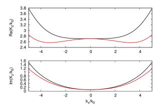
FIG. 3. Dispersion curves for a metallo-dielectric structure  $(h_d = 5 \text{ nm}, h_m = 22.6 \text{ nm}, \lambda = 363.8 \text{ nm})$  in the canalization regime (*i.e.* a flat dispersion curve). Top: Real part. Bottom: Imaginary part. The local (black line) and nonlocal (red line) cases are shown. The difference is much more important here: nonlocality has a direct impact on the curvature of the dispersion curve.
