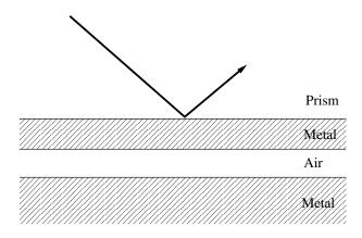
FIG. 8. Diagram of the excitation of a gap-plasmon using a prism coupler. The thickness of the upper metallic layer is 18 nm.
