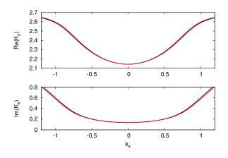
FIG. 2. Dispersion curves for a metallo-dielectric structure  $(h_d = 33.7 \text{ nm}, h_m = 28.1 \text{ nm}, \lambda = 363.8 \text{ nm})$  presenting an effective index close to -1. Top: Real part. Bottom: Imaginary part. The local (black line) and nonlocal (red line) cases are shown. Very little difference can be seen, especially close to normal incidence.
