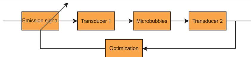
1. Transmit pulse with the frequency  $f_{old}$  and a 4 cycles  $\rightarrow$  Constant transmit power
