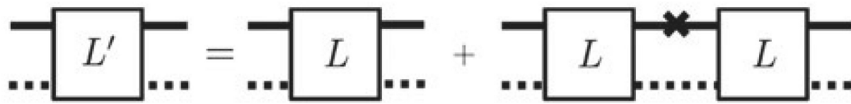
Figure 3. Diagrammatic representation of the modified Ladder operator L' . The solid (resp. dashed) horizontal lines represent the average retarded (resp. advanced) Green's function \overline{G}^+ (resp. \overline{G}^- ) and the cross represents the T -matrix of the new scatterer appearing in the medium. Here we assume that the new scatterer is far enough from the source and the receiver (a few \ell ).
