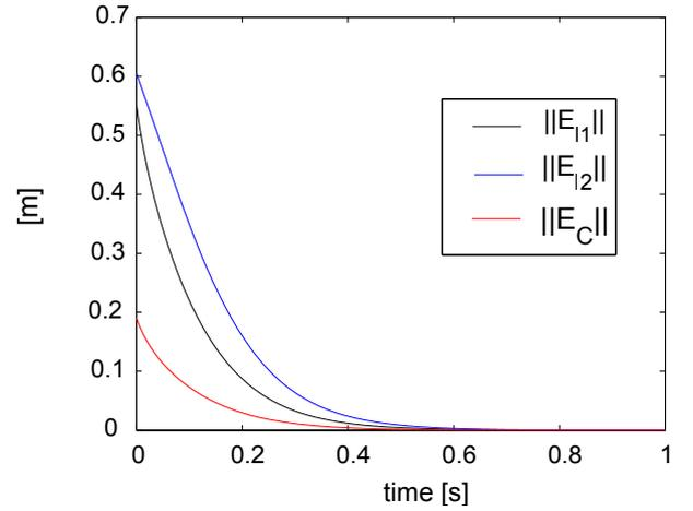
(b) Errors of the line-based controller.
