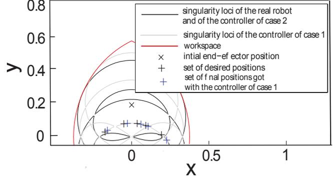
Figure 8: Singularity loci of the five-bar mechanism and its corresponding hidden robot for the following set of parameters:  $l_{1i} = 0.3$  m,  $l_{2i} = 0.35$  m,  $l_{OA_i} = 0.275$  m.
