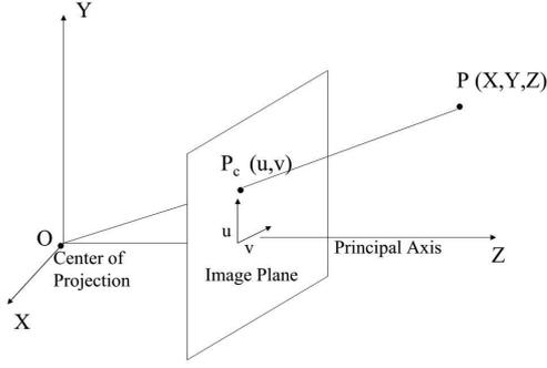
Figure 9: A pinhole camera model
