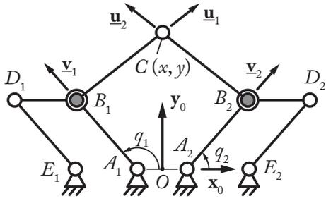
Figure 5: The hidden robot involved into the leg-direction-based visual servoing approach of the five-bar mechanism (the gray pairs denote the actuated joints)
