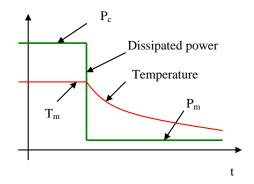
Fig. 2. Temperature measurement using a low calibration power P<sub>m</sub>
