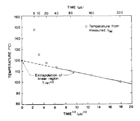
Fig. 3. Device temperature measurement of a bipolar transistor [30]
