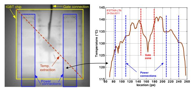
Fig. 1. Infrared imaging of a functioning IGBT chip
