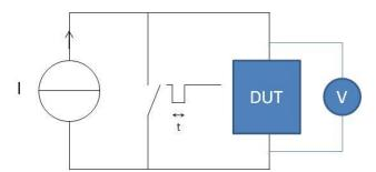
Fig. 9. Electrical circuit for the calibration step with a high current injected in the device
