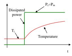
Fig. 4. Temperature measurement using a high calibration power Pm
