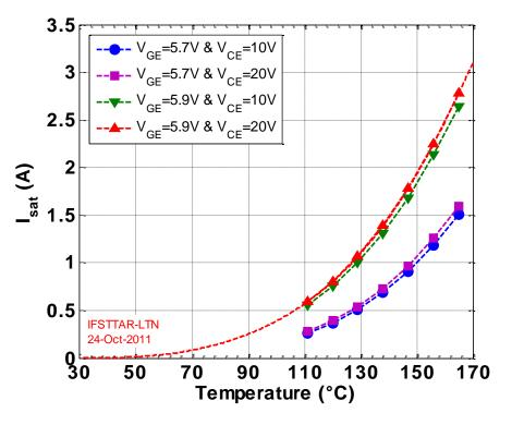
b. I<sub>sat</sub> value as a function of temperature
