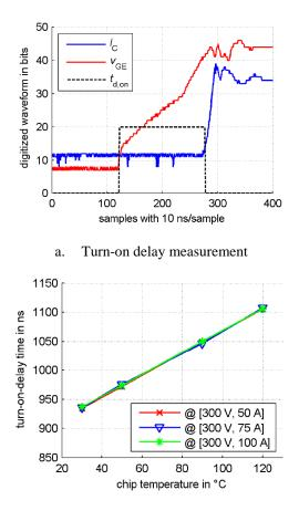
b. Turn-on delay as a function of temperature
