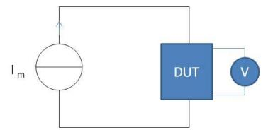
Fig. 5. Calibration step with a low current injection
