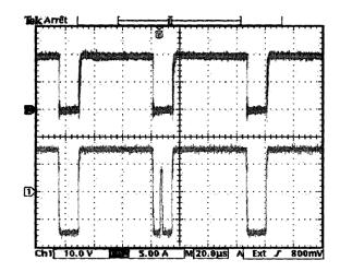
Fig. 14. Gate-emitter voltage (channel 1) and collector current (channel 2) for an IGBT on-line temperature measurement using the saturation current as a thermo-sensitive parameter [50]
