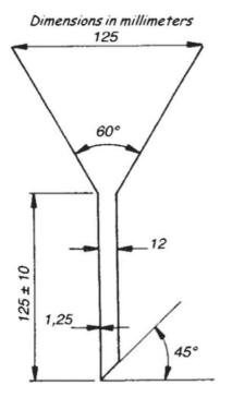
Fig. 1. Dimensions of the funnel used for measuring the flowability.
