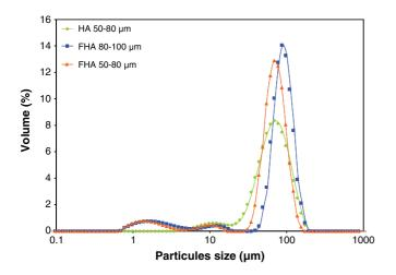
Fig. 4. Particle size distributions of the powders: FHA 80–100µm, FHA 50–80µm and HA reference powder.
