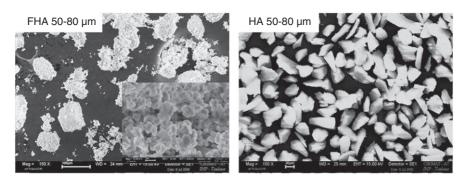
Fig. 5. SEM micrographs of the FHA sieved between 50 and 80µm and the reference HA powder (50-80µm).
