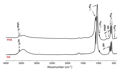
Fig. 3. FTIR spectra of the as-synthesized fluor-hydroxyapatite powder and hydroxyapatite reference powder.
