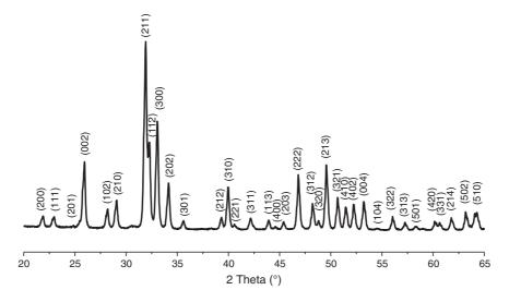
Fig. 2. X-ray diffraction diagram of the synthesized FHA powder.
