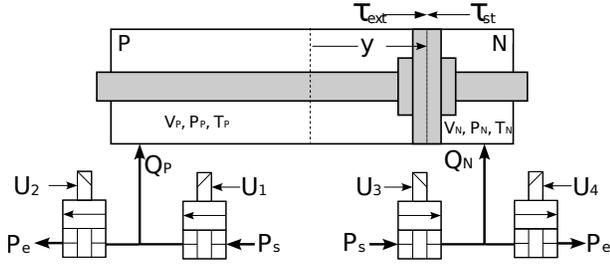
Fig. 1. A pneumatic actuator with 4 on/off solenoid valves.
