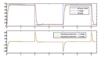
Fig. 6. PWM tracking of the actuator for a square input.
