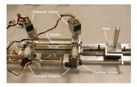
Fig. 4. Experimental setup.
