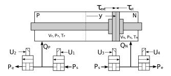
Fig. 1. A pneumatic actuator with 4 on/off solenoid valves.
