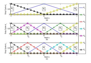
Fig. 3. Duty cycle mapping for: (a) the 3-mode system, (b) the 5-mode system or 7-mode system (pressurizing profile), or (c) the 7-mode system (venting profile).
