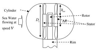
Fig. 7. Representation of a stator inserted in a cylindrical nozzle.
