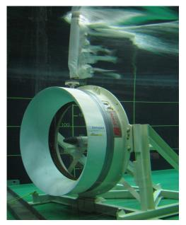
Fig.2. Rim-driven prototype integrating a RFPM machine [8].
