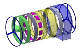
Fig 1. Principle of a rim-driven turbine
