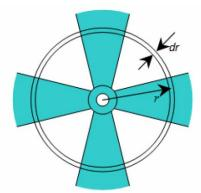
Fig. 7: radial split of the turbine disk in disk element.
