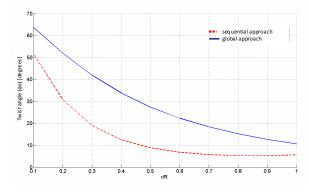
Fig. 10 : Twist law of the two blade designs as a function of the reduced radius (r/R)
