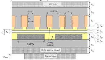
Fig. 4. Main dimensions of the electrical machine
