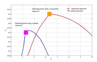
Fig.9 : Power coefficient,  $C_p$ , versus tip speed ratio ( $\lambda$ =TSR= $2\pi$ RN/( $60.V_o$ )) of the two designed turbines (hydrodynamic characteristic only)
