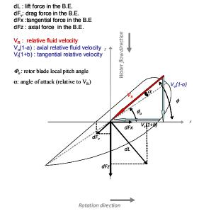
Fig.8: Forces and water relative water speed in a blade element
