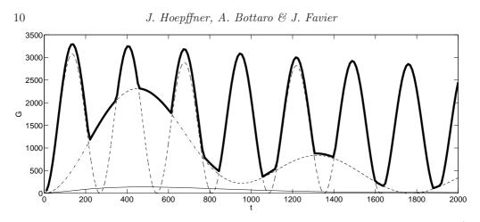
FIGURE 4. Thick line: envelope of maximum energy growth for  $(\alpha, \beta) = (0, 0.2)$ ,  $K = 10^4$ , Re = 5000, d = 1. We observe two oscillatory behaviours with *apparent* periods  $T \approx 270$  and  $T \approx 950$ . The energy evolution of the initial conditions optimal for t = 400 and t = 500 are represented with dashed and dot-dashed lines. The optimal growth envelope for the rigid channel at Re = 5000 is drawn with a thin solid line.
