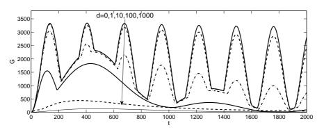
FIGURE 6. Effect of wall damping on energy growth. Parameters as by figure 4, with d = 0, 1, 10, 100, 1000. The optimal growth envelope for the rigid channel is drawn with a thin solid line.
