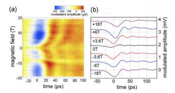
FIG. 2: (a) 3D colour plot of modulated signal amplitude in the propagation time - magnetic field plane. (b) Five signals chosen at filling factors  $\nu=2,6,10$ , offset for clarity. From top to bottom: 18T, 6T, 3.6T, 0T, -3.6T, -6T, -18T. These data correspond to 11ps excitation and 5ps sampling resolution.
