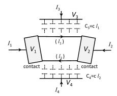
FIG. 9: **Two ohmic contacts.** Conductance between two ohmic contacts connected with two chiral states of lengths  $l_1$  and  $l_2$ .
