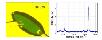
FIG. 4: Raman sample characterisation. (a) Raman map of the sample, where green corresponds to graphene. (b) Raman spectrum in the middle of the graphene sample.
