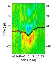
FIG. 5: **Field derivative of the transmitted signal.** Rainbow colour plot of the derivative of the transmitted signal with respect to the magnetic field. Positive to negative values range across the spectrum from red to blue. The black and red superimposed data points are the transmitted pulse arrival times as shown in Figure 3 of the main text, where the signal is modulated with respect to gate voltage.
