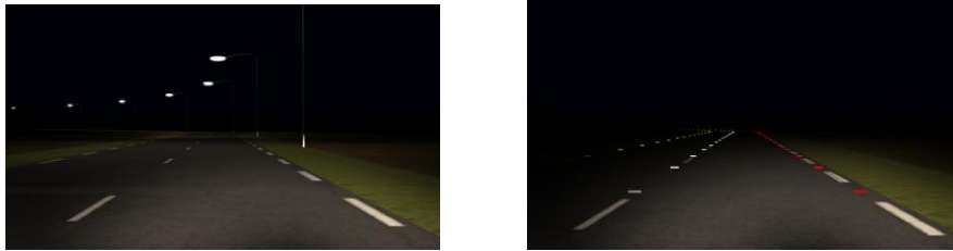
Fig. 4. High Dynamic Range rendering of night-time driving conditions with road lighting (left) and LED studs (right).
