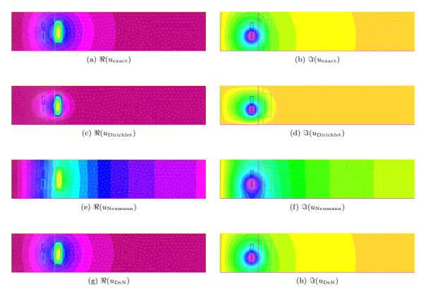
Figure 6: Real and imaginary parts of u fields of the truncated model with different boundary conditions. DtN maps of truncation order N = 20.
