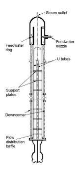
Figure 1: Sketch of a steam generator.
