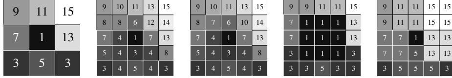
Fig. 7. From left to right: an image, and its interpolations with the median , the mean/median , the min and the max .
