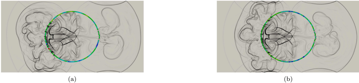
Figure 12: Density field in the fluid and normal stress distribution in the cylinder discretized with (a) 100 particles and (b) 200 particles at time 24.4ms.
