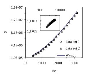
**Figure 2:** Viscous torque of the inner cylinder in single-phase flow measured as a function of the Reynolds number for a mixture of 65% glycerol. Comparison with Wendt's correlation (1933).
