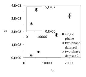
**Figure 5:** Viscous torque of the inner cylinder measured as a function of the Reynolds number for a mixture of 40% glycerol,  $\Phi_c=20\mu m$ , P=6b, 1h30 after stabilizing the rotational velocity. Comparison with single phase-flow.
