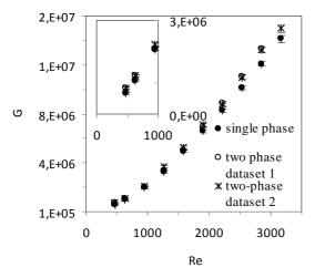
**Figure 4:** Viscous torque of the inner cylinder measured as a function of the Reynolds number. for a mixture of 65% glycerol,  $\Phi_c=180\mu$ m, P=1.08b. 50 mn after stabilizing the rotational velocity. Comparison with single-phase flow.
