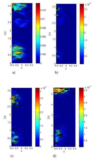
**Figure 9:** Void fraction distribution measured in a meridian plane by bubbles tracking for the different cases a, b, c and d.
