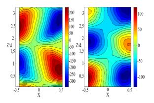
**Figure 12:** Axial component of the mean liquid velocity measured in a meridian plane by PIV (left : single phase, right : two-phase case a)
