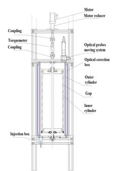
Figure 1: Sketch of the experimental setup.
