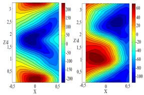
**Figure 13:** Radial component of the mean eulerian liquid velocity measured in a meridional plane by PIV (left : single phase, right : two-phase case a)
