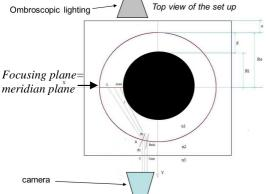
Figure 8: Top view of the set up for bubbles tracking.
