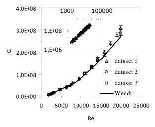
**Figure 3:** Viscous torque of the inner cylinder in single-phase flow measured as a function of the Reynolds number for a mixture of 40% glycerol. Comparison with Wendt's correlation (1933).
