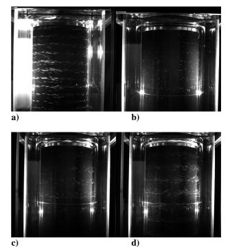
**Figure 6:** Visualisations of the two-phase flow arrangement for the different cases a to d. Traces of the bubbles are visible for several wavelengths over the height of the device by integrating with an exposure time of 20ms.
