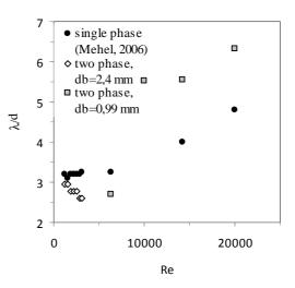
**Figure 7:** Axial wave length measured as a function of the Reynolds number for the different mixtures and bubble sizes. Comparison with single- phase flow is also added based on Mehel's measurements (2006) (Note that for Re=10000, Mehel didn't evidence very clear Taylor vortices in single phase flow).
