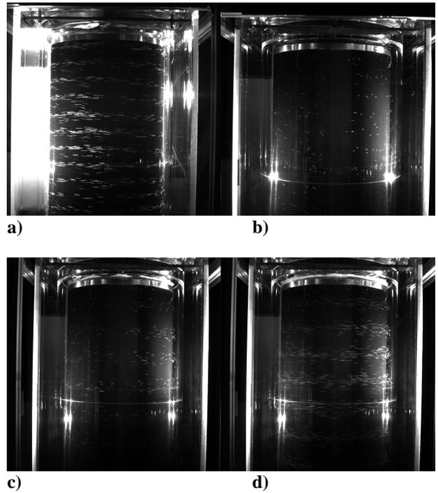
**Figure 6:** Visualisations of the two-phase flow arrangement for the different cases a to d. Traces of the bubbles are visible for several wavelengths over the height of the device by integrating with an exposure time of 20ms.
