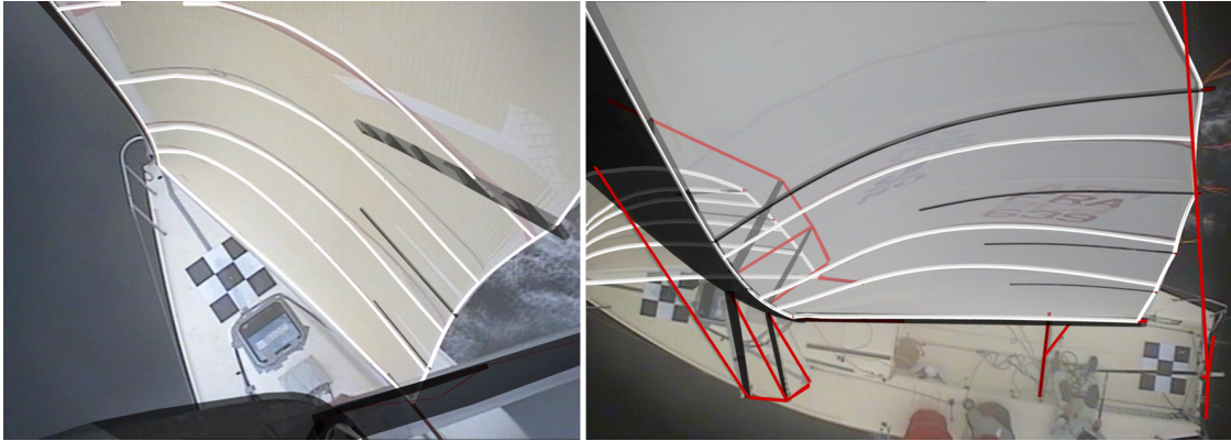
Figure 19: Comparison of the experimental flying shape and the numerical result on a port tack close hauled steady state. The picture and gray visualisation stripes show the measured flying shape; the black thick lines show the computed position of the beams in the model (mast, boom, spreaders, battens); the white lines show the computed sails outline and visualisation stripes
