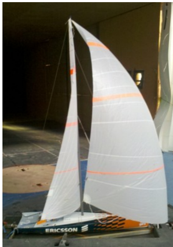
Figure 4: VO70 model scale yacht used for the FEPV wind tunnel validation where the VSPARS calculated sail positions were compared with physical measurements
