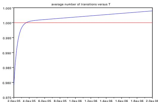
Figure 1: Average number of transitions. We set  $\epsilon = 0.1$ ,  $V = 2$ ,  $v = 1$ ,  $p = q = 1$  and let  $T$  vary. We compute numerically the average number of transitions per period. We can clearly observe that there is one and only one period corresponding to the condition (3.5).
