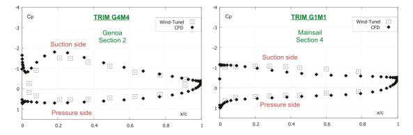
**Fig. 5.** Cp on Section 2 of the genoa for the loosest mainsail and genoa trim (G4M4), which corresponds to the minimum flow separation.
