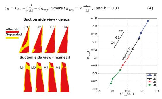
**Fig. 16.** Attached and separated flow areas on the suction side of the sails: four genoa trims for the mainsail trim M2 and four mainsail trims for the genoa trim G3 (maximum  $C_x$  is achieved for M2G3)
