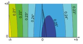
**Fig. 7.** Contours of the velocity magnitude increase on the jet section.
