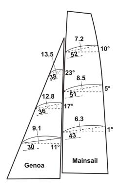
**Fig. 9.** Breakdown of the aerodynamic force and effect of a trim variation.
