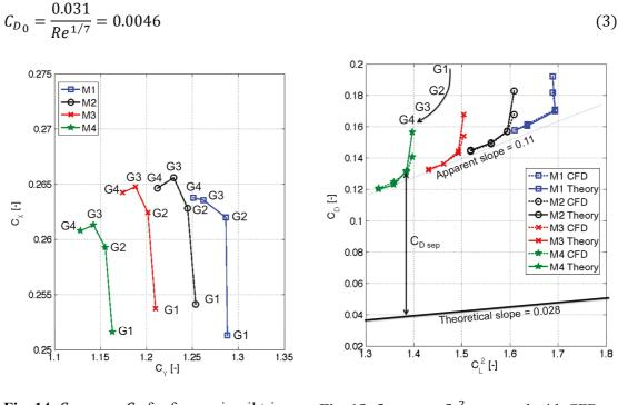
**Fig. 14.**  $C_x$  versus  $C_y$  for four mainsail trims (M1-4) and four genoa trims (G1-4).
