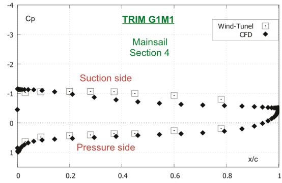
**Fig. 6.**  $C_p$  on Section 4 of the mainsail for the tightest mainsail and genoa trim (G1M1), which corresponds to the maximum flow separation.
