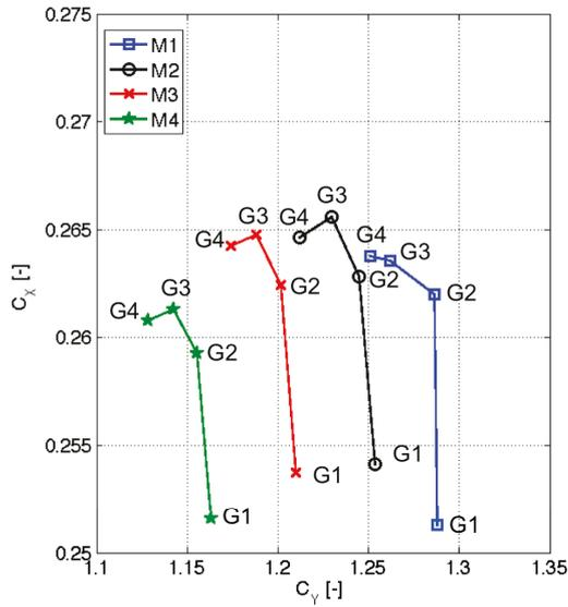
**Fig. 14.**  $C_x$  versus  $C_y$  for four mainsail trims (M1-4) and four genoa trims (G1-4).
