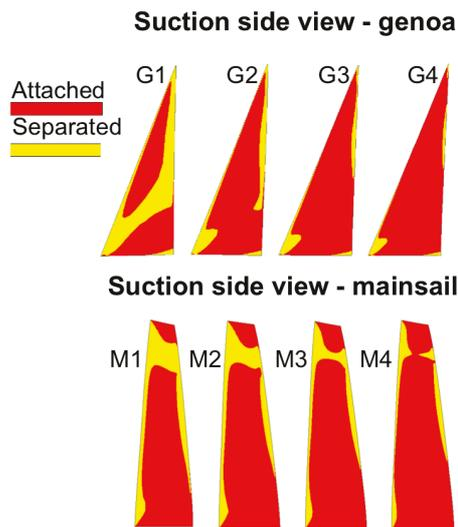
**Fig. 16.** Attached and separated flow areas on the suction side of the sails: four genoa trims for the mainsail trim M2 and four mainsail trims for the genoa trim G3 (maximum  $C_x$  is achieved for M2G3)
