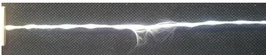
Fig. 5. GFPP yarn after breaking
