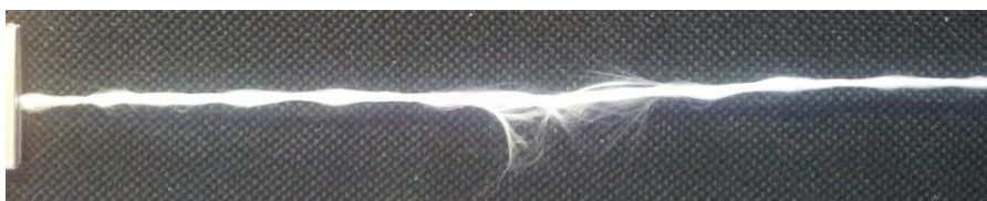
Fig. 5. GFPP yarn after breaking
