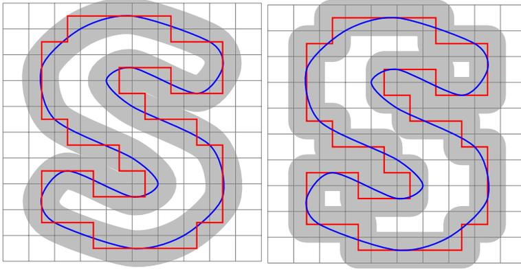
FIGURE 4. Illustration of the fact that the boundary of  $X$  and the  $h$ -boundary of  $X$  are Hausdorff close, with distance no greater than  $\frac{\sqrt{d}}{2}h$ . On the left,  $\partial_h X$  lies in the  $\frac{\sqrt{d}}{2}h$ -offset of  $\partial X$  (in gray). On the right,  $\partial X$  lies in the  $\frac{\sqrt{d}}{2}h$ -offset of  $\partial_h X$  (in gray).
