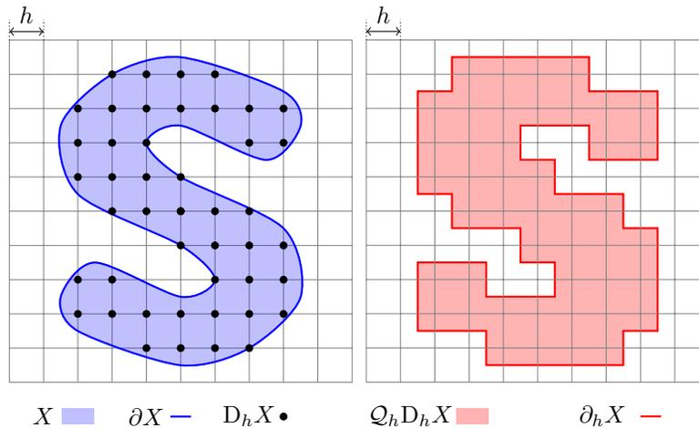
FIGURE 1. Illustration of the main definitions used throughout the paper: a shape  $X$ , its boundary  $\partial X$ , its Gauss digitization  $D_h X$ , its  $h$ -cube embedding  $\mathcal{Q}_h D_h X$  and its  $h$ -boundary  $\partial_h X$ .
