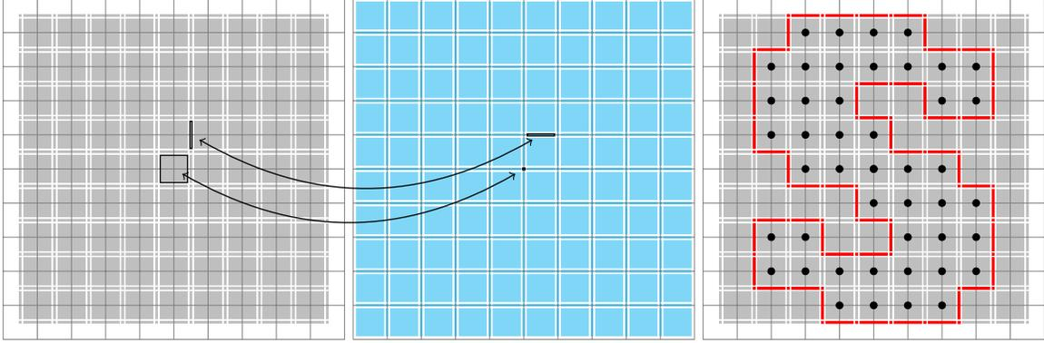
FIGURE 3. Illustration of (left) the primal cubical grid  $\mathbb{F}_h$  in gray, (middle) the dual cubical grid  $\tilde{\mathbb{F}}_h$  in cyan, (right) the Gauss digitization  $D_h X$  in black and the  $h$ -boundary of  $X$  in red, seen as a subcomplex of  $\mathbb{F}_h$ . Note that some cells and their dual are shown between the two grids.
