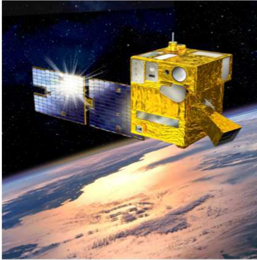
Figure 1. (left) PICARD is a spacecraft dedicated to simultaneous measurement of the solar radius, the solar shape, the solar irradiance and the solar interior. The payload consists of two absolute radiometers (provided by Royal Meteorological Institute of Belgium (RMIB) and by Physikalisch Meteorologisches Observatorium of Davos (PMOD)) measuring the TSI, and a Ritchey-Chrétien imaging telescope to determine the solar radius and asphericity (LATMOS). (right) “PICARD SOL” (under the responsibility of Observatoire de la Côte d’Azur (OCA) and LATMOS) is a set of instruments based at the Calern site (Observatoire de la Côte d’Azur, France) to carry out solar radius with the capability in discriminating as much as possible the measurements affected by atmospheric effects. A replica of the space instrument was installed at the Calern observatory, which provides a nearly continuous record of the solar radius at different wavelengths since May 2011. The picture corresponds to the telescope equatorial mount. The replica of the space telescope is placed in a vacuum tank closed by a glass window.
