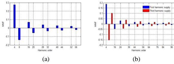
Fig. 7. MMF spectrum .(a) 12/8/3 machine ; (b) 20/8/5 machine.
