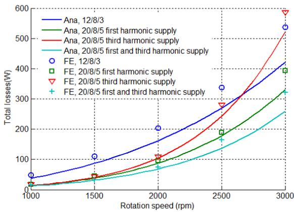
Fig. 11. Total losses in the two machines.
