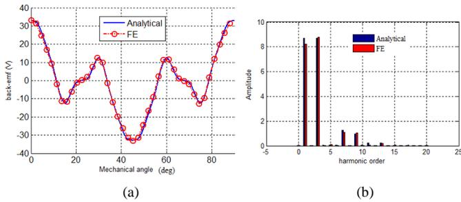
Fig. 3. (a) Back-emf for 20/8/5 machine . (b) Harmonic content of back-emf
