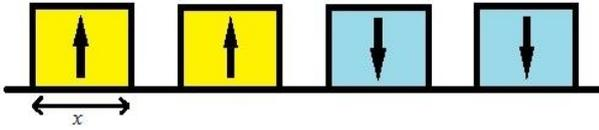
Fig. 2. Magnet layer of 20/8/5 machine .
