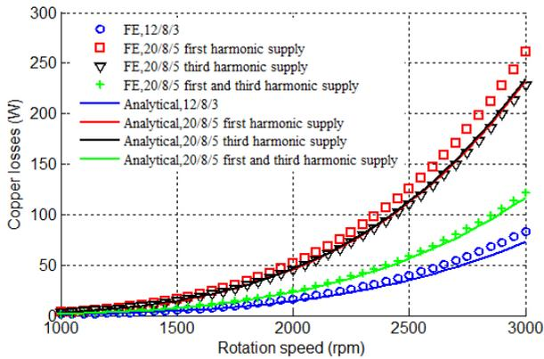
Fig. 5. Copper losses in the two machines 20/8/5 and 12/8/3.
