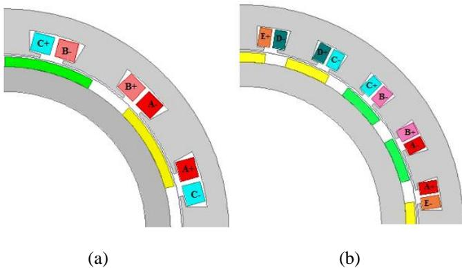
Fig. 4. (a) 12/8/3 machine . (b) 20/8/5 machine.
