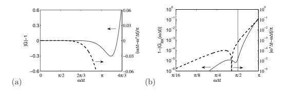
Figure 19: Properties of schemes in the frequency space  $\omega \Delta t$ . Amplication rate (------) and phase error (-----) of the optimized Runge-Kutta scheme on linear scale (a) and on logarithmic scale (b). Low-storage fourth-order Runge-Kutta of Bogey and Bailly [38] with 6 sub-steps.
