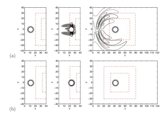
Figure 23: Isocontours of the instantaneous pressure disturbance at three successive instants,  $N_{it} = 100, 200, 350$  (from left to right), showing the passage of the vortex through the first overset interface (--). Lagrange interpolations are used on a  $2 \times 2$  (a) and  $6 \times 6$  (b) stencil. Isocontours values are  $\pm 1$  Pa, and  $\pm 5$  to  $\pm 20$  Pa with step of 5 Pa.
