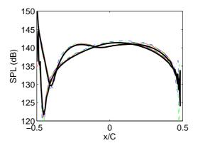
Figure 36: Unsteady pressure distribution over the vane at the first harmonic: (----) present simulation, (-----) Coupland [48], (----) Nallasamy *et al.* [43] (-2.5dB), (----) Wang *et al.* [49] (+4dB).
