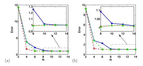
Figure 27: Normalized error for a source of pulsation  $\omega = 2\pi/5 \times c_{\infty}/\Delta x$ . Same legend as figure 25: (a) foreground Cartesian grid, (b) foreground sinusoidal grid.
