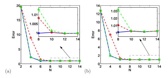
Figure 26: Normalized error for a source of pulsation  $\omega = 2\pi/10 \times c_{\infty}/\Delta x$ . Same legend as figure 25: (a) foreground Cartesian grid, (b) foreground sinusoidal grid.
