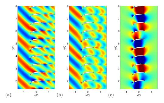
Figure 35: Gust-cascade interaction tone at the first BPF frequency: instantaneous perturbations of the longitudinal velocity u' (a), of the transverse velocity v' (b), and of the pressure p' (c). Colormap bounds are  $\pm 2$  m/s for the velocity maps, and  $\pm 200$  Pa for the pressure.
