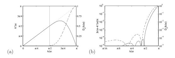
Figure 18: Properties of schemes in the wavenumber space  $k\Delta x$ . (a) The effective wavenumber  $k^*\Delta x$  of the eleven-point-stencil optimized scheme (-----), and the damping function  $D_k(k\Delta x)$  of the eleven-point stencil optimized filter (------). (b) The dissipation errors  $|k\Delta x - k^*\Delta x|/\pi$  for the discretization schemes and  $D_k(k\Delta x)$  for the optimized filter are shown on a logarithmic scale.
