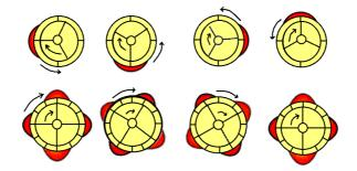
Figure 34: Rotor-Stator interaction with 3 blades and 4 vanes (first row), and 4 blades and 12 vanes (second row). The red lobes mark the acoustic pulses when a blade and a vane are coincident, forming a circumferencial mode. The arrows indicate the direction of rotation of the rotor and of the generated pressure waves.
