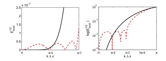
Figure 6: Comparison of the local error in the wavenumber space, obtained with Lagrange interpolation (----) and optimized interpolation (----), for N = 8.
