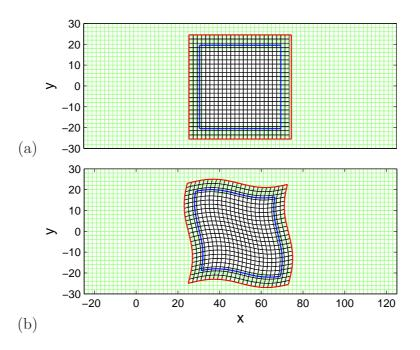
Figure 22: Overlapping of a Cartesian grid (---) by another Cartesian grid (a), or a sinusoidal grid (b) (---). Every two points are represented. The grid with the higher priority is the foreground grid, so that the cutting hole process is applied to the background grid.
