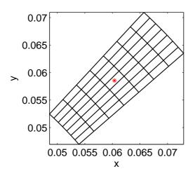
Figure 14: Curvilinear 8×8 stencil used for the spectral analysis of 2-D interpolation methods;  $\Delta r=0.0036$ , and  $\Delta \theta=2\pi/410$ .
