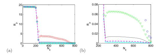
Figure 24: Temporal evolution of the residual pressure  $R_p$ , eq.(35). (a) Stencils  $2 \times 2$  ( $\Box$ ),  $4 \times 4$  (o),  $6 \times 6$  ( $\nabla$ ). (b) Close-up view where the results for stencils  $8 \times 8$  (--),  $10 \times 10$  (---),  $12 \times 12$  (---\*) have been added. The Cartesian foreground grid is used with Lagrange interpolations.
