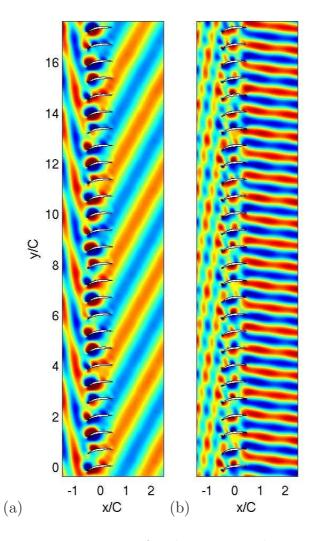
Figure 37: Acoustic rotor-stator tones for the 27 vanes domain. Instantaneous pressure disturbances at the second harmonic (a) with levels  $\pm 50$  Pa, and at the third harmonic (b) with levels  $\pm 12.5$  Pa.
