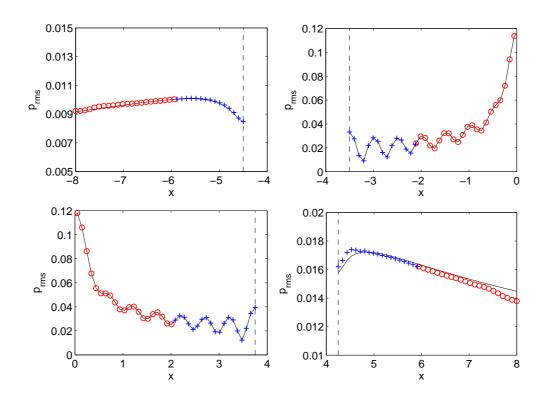
Figure 29: Root mean square pressure along y = 0: analytical solution (------), numerical solution for the two polar grids (+) and the Cartesian grid ( $\circ$ ). The vertical dashed lines depict the location of the cylinder boundaries. The first two plots are upstream and downstream of the cylinder located at x = -4 m, and the two last plots show the rms pressure upstream and downstream of the second cylinder at x = 4 m.
