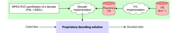
Figure 8: Conceptual process of an RVC decoder implementation.
