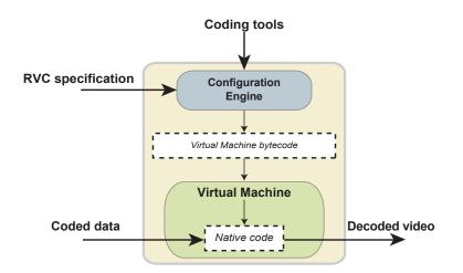
Figure 13: Reconfigurable implementation of MPEG RVC decoder based on virtual machines.
