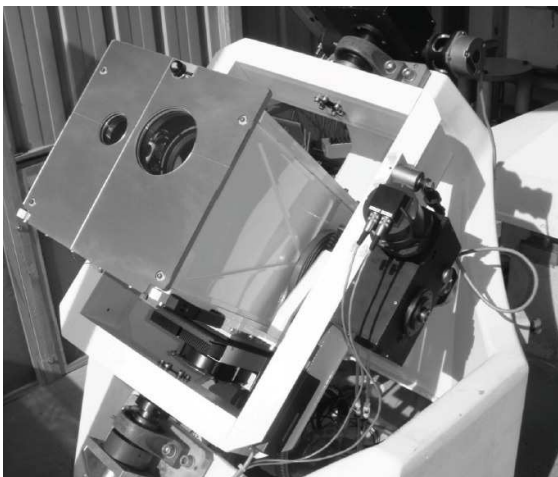
Fig. 3. View of the SODISM II equatorial mount. The ground-based telescope is placed in a vacuum tank closed by a glass window.
