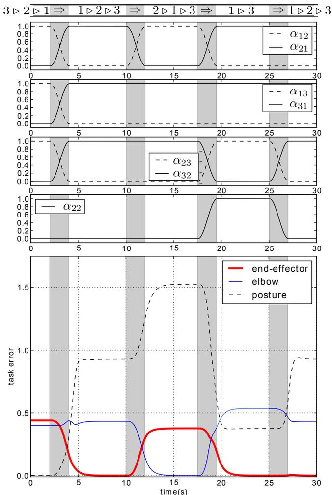
Fig. 9: Evolution of  $\alpha$ s (top) and task errors (bottom) using GHC, with fixed task targets. Priority transitions as well as the insertion and deletion of the elbow task are performed. Strict priorities are well respected and the error of the highest priority task is maintained at 0 during steady states.
