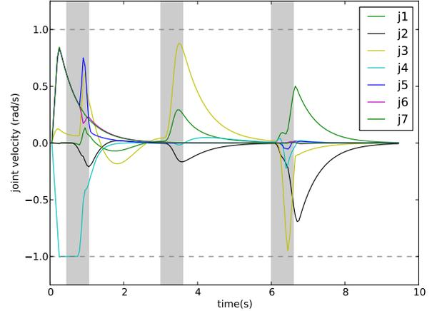
Fig. 4: Evolution of the joint velocities. The upper and lower bounds of  $\dot{q}$  are  $1 \text{ rad/s}$  and  $-1 \text{ rad/s}$ , respectively. These bounds are voluntarily set low in order to easily illustrate the fact that they are respected.
