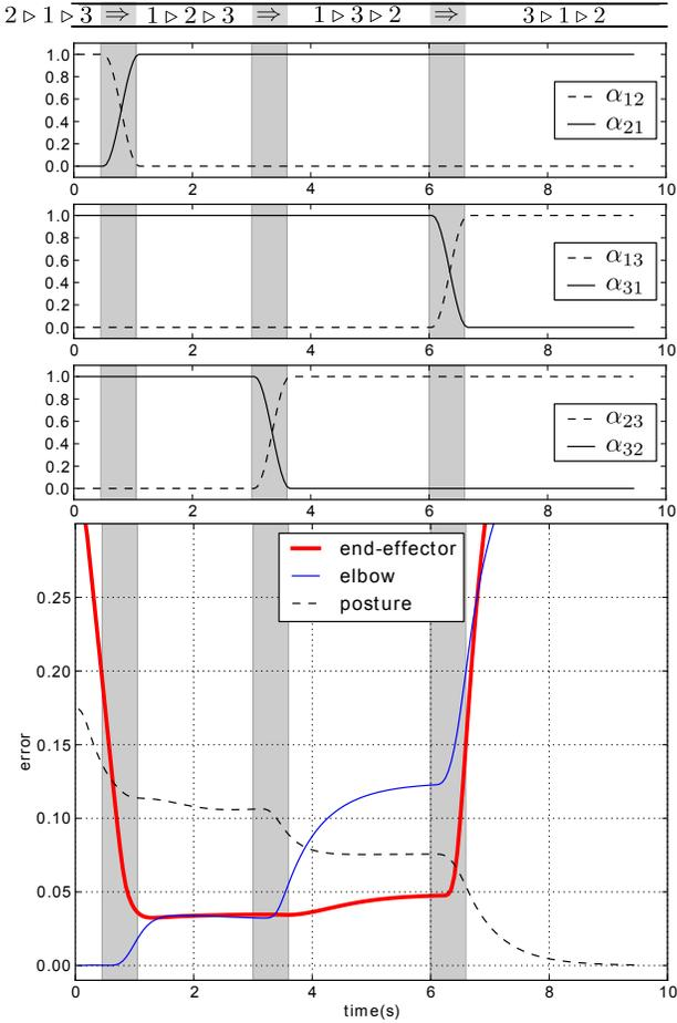
Fig. 2: Evolution of  $\alpha_s$  (top) and task errors (bottom) during priority switching subject to constraints. Task priorities are switched continuously with the continuous change of  $\alpha_s$ . The end-effector task error is not decreased to 0 when its task priority is the highest: the obstacle avoidance constraint is respected, and the end-effector cannot arrive at its target position behind the obstacle plane.
