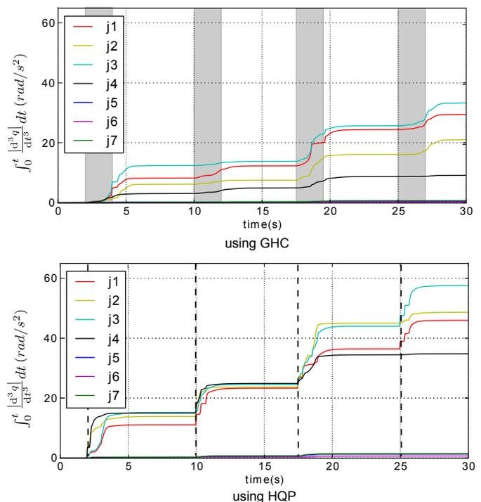
Fig. 11: Integration of the absolute values of joint jerks using GHC (top) and HQP (bottom), with fixed task targets. GHC generates smaller joint jerks than HQP does, while the latter one provides larger jerks each time task hierarchy is changed.
