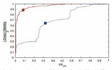
**Fig. 11.** Results of the bearing fault detection on campaign 1 in terms of false alarms, delay and stability with different threshold values for energy-based (dashed blue) and statistic-based indicators (plain red). The optimal points are pictured as a box and a star respectively. (For interpretation of the references to color in this figure caption, the reader is referred to the web version of this paper.)
