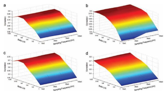
Fig. 10. Correlation results of the statistic-based indicator for different window sizes and sampling frequencies at 8000 rpm (a), 10,000 rpm (b), 12,000 rpm (c) and 14,100 rpm (d).
