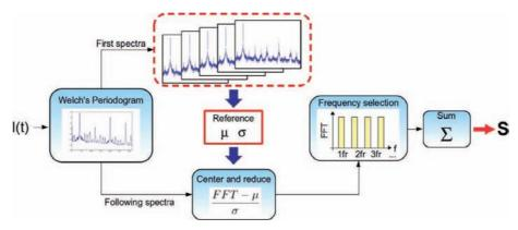
Fig. 8. Principle of the statistic-based method.
