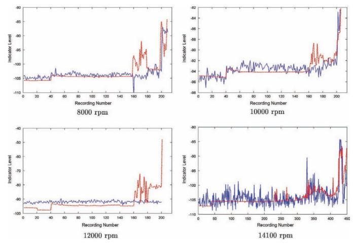
**Fig. 13.** Energy-based indicators (plain blue line) and vibration indicators (dotted red line) obtained on campaign 2 at different speeds. (For interpretation of the references to color in this figure caption, the reader is referred to the web version of this paper.)
