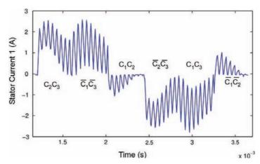
Fig. 3. Example of stator current I1 on phase 1 generated by the PWM.
