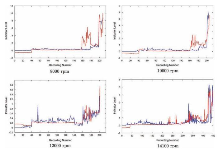
**Fig. 15.** Statistic-based indicators (plain blue line) and vibration indicators (dotted red line) obtained on campaign 2 at different speeds. (For interpretation of the references to color in this figure caption, the reader is referred to the web version of this paper.)
