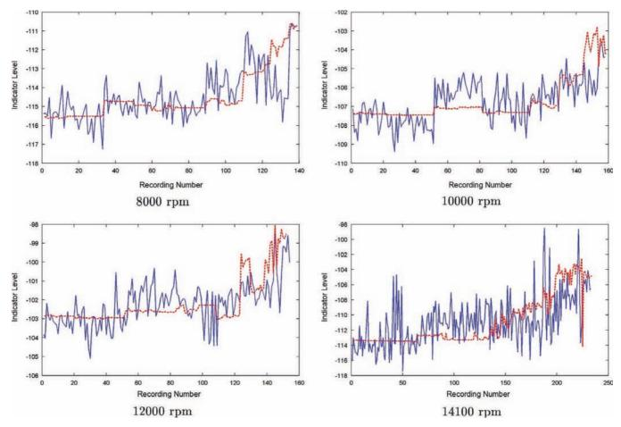
**Fig. 12.** Energy-based indicators (plain blue line) and vibration indicators (dotted red line) obtained on campaign 1 at different speeds. (For interpretation of the references to color in this figure caption, the reader is referred to the web version of this paper.)
