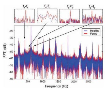
**Fig. 5.** Stator current spectrum in faulty (red plain line) and healthy (blue line) cases at 12,000 rpm. (For interpretation of the references to color in this figure caption, the reader is referred to the web version of this paper.)
