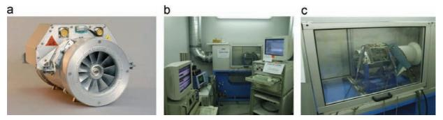
Fig. 1. (a) TECHNOFAN LP2 fan, (b) and (c) bearing fault diagnostic experimental test bench.
