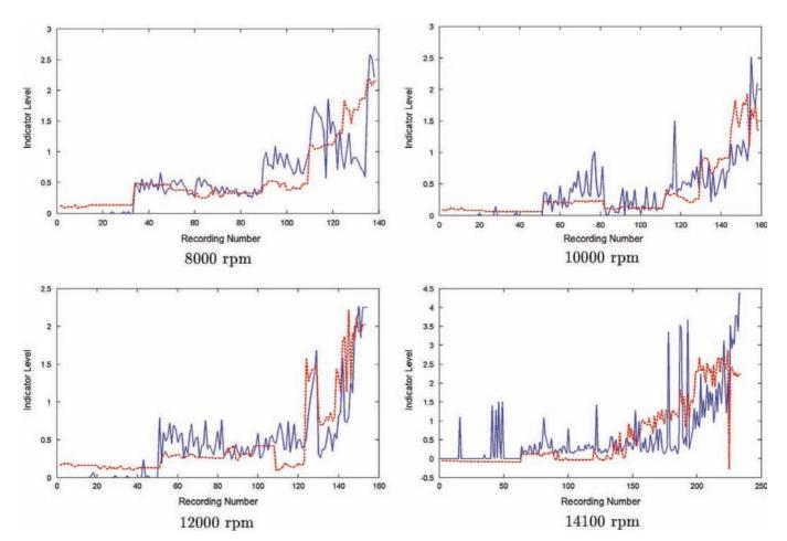
**Fig. 14.** Statistic-based indicators (plain blue line) and vibration indicators (dotted red line) obtained on campaign 1 at different speeds. (For interpretation of the references to color in this figure caption, the reader is referred to the web version of this paper.)
