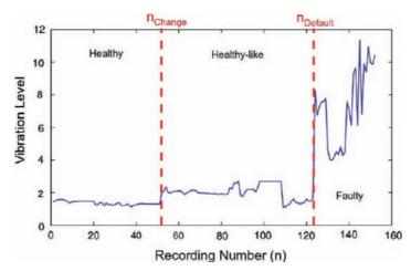
Fig. 9. Example of the markers  $n_{Change}$  when the bearing is replaced by a faulty one and  $n_{Default}$  when the vibration indicator starts reacting.
