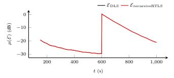
Fig. 11. Squared error vector norm averaged over 500 independent noise realizations for right noise covariance matrix  $(P_r)$  scenario Ne4 of Tab. II. Contrary to all previous results, the true inputs  $(\overline{A})$  were built from white Gaussian noise with zero mean and unit variance.
