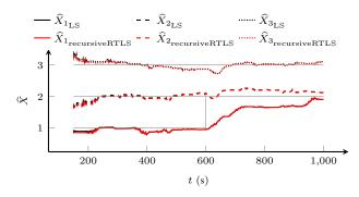
Fig. 5. Estimated parameter vector  $(\hat{X})$  of one experiment for right noise covariance matrix  $(P_r)$  scenario No3 of Tab. II. The true parameters  $(\overline{X})$  are shown by —.
