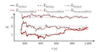
Fig. 2. Estimated parameter vector  $(\widehat{X})$  of one experiment for right noise covariance matrix  $(P_r)$  scenario No1 of Tab. II. The true parameters  $(\overline{X})$  are shown by —.
