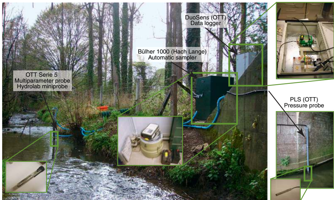
Fig. 7. Monitoring station placed at the outlet of the Lingèvres catchment.
