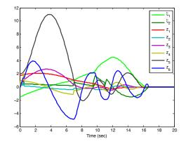
Fig. 1. The convergence of the extended chained form system starting from the initial state  $x_0 = [-1.5, 0, 1.75, 0, 0.5, 0, 2, 0]^T$  and converging to a final desired state  $x_d = [0, 0, 0, 0, 0, 0, 0, 0]^T$  with the saturation constraints on the control inputs  $[u^{max}, v^{max}] = [5, 5]$  and  $q_{max} = 2$  with  $\delta = 0.1$  sec.
