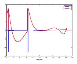
Fig. 4. The control inputs u (in blue) and v (in red) applied for steering the extended chained form system from a singular initial state  $\mathbf{x}_0 = [0, 0, 1.75, 0, 0.5, 0, 2, 0]^T$  to a final desired state  $x_d = [0, 0, 0, 0, 0, 0, 0, 0]^T$  with the saturation constraints on the control inputs  $[u^{max}, v^{max}] = [5, 5]$  and  $q_{max} = 2$  with  $\delta = 0.1$  sec.
