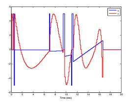
Fig. 2. The control inputs u (in blue) and v (in red) applied for steering the extended chained form system from the initial state  $x_0 = [-1.5, 0, 1.75, 0, 0.5, 0, 2, 0]^T$  to a final desired state  $x_d = [0, 0, 0, 0, 0, 0, 0, 0]^T$  with the saturation constraints on the control inputs  $[u^{max}, v^{max}] = [5, 5]$  and  $q_{max} = 2$  with  $\delta = 0.1$  sec.
