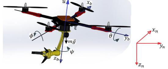
Fig. 2. Schematic configuration of a quadrotor carrying a manipulator arm.
