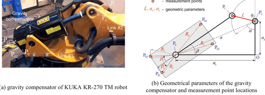
(a) gravity compensator of KUKA KR-270 TM robot
