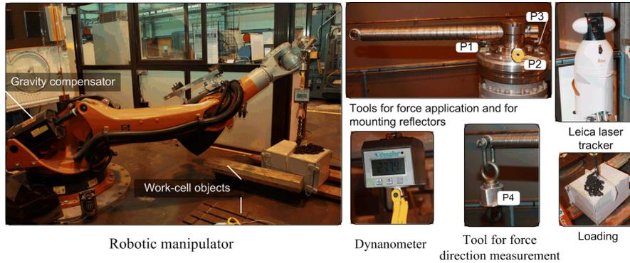
**Fig. 3** Experimental setup for manipulator elastostatic calibration
